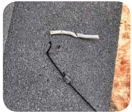
A vinyl coated, stainless steel tie cinched so tight that it cut through the wire. Photo source: PV Pros, Inc.
