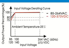
Note: ①With an input voltage between 85-100VAC and a DC input between 120-140VDC the output power must be derated as per the temperature derating curves:
