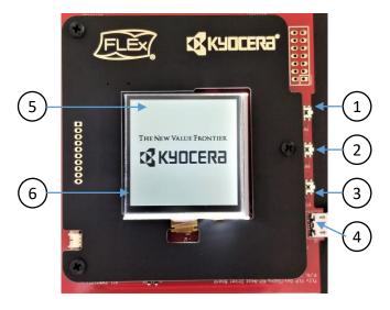
• Note: The optical surface underneath the protective film is very delicate and will be permanently marked by fingerprints. Use care when removing it with the blue pull tab.
