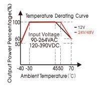
Note: With an AC input voltage between 90-100VAC and a DC input between 120-141VDC the output power must be derated as per the temperature derating curves.
