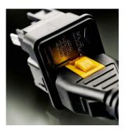
Unlike wire bail or clamp accessories, no additional costly hardware is necessary to install the cord retaining system. The cord set safely latches into a notch in the plastic housing of the KEA. Removing the cord set is easily achieved by depressing the latch. V-Lock power cords are offered in a wide range of international plugs, including NEMA 5-15 standard hospital grade versions.
