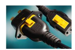
The new V-Lock power cord provides a safe and reliable power connection. It conveniently latches into the notched inlet or outlet to prevent accidental disconnection of the power from the equipment. The yellow catch mechanism is easily released by depressing the lever. Unlike wire bail or clamp accessories, no additional hardware is required to install the cord retaining system, saving installation time and material.
