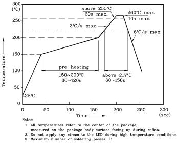
Reflow Soldering Profile for SMD Products (Pb-Free Components)
